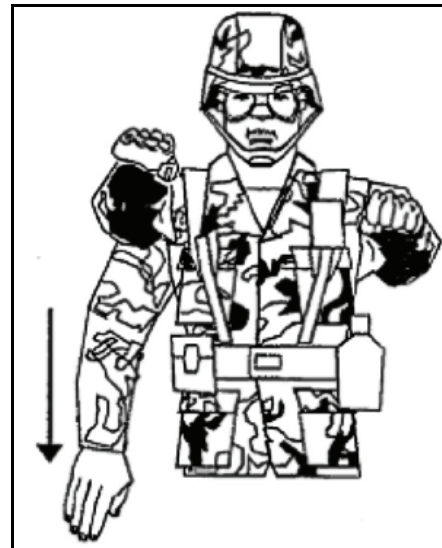
Figure A-41. Winch down Extend left arm horizontally in front of body with fist clenched; extend right arm forward with palm turned down and make a downward motion.
