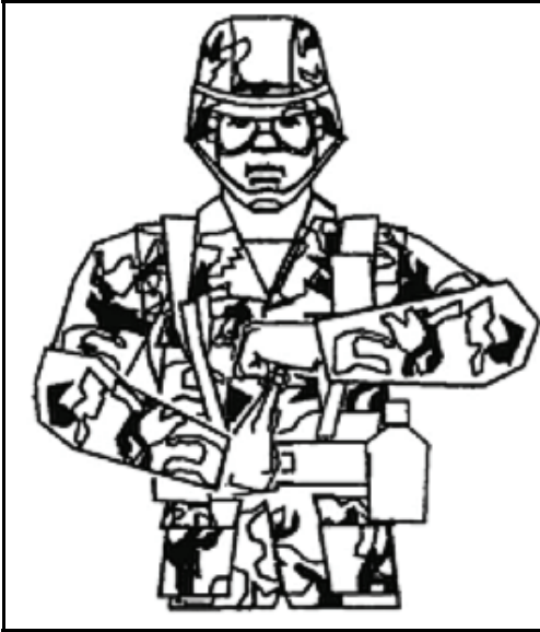
Figure A-38. Load has not been released Bend left arm horizontally across chest with fist clenched and palm turned down; open right hand pointed up vertically to center of left fist.
