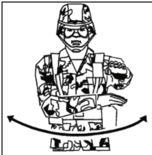
Figure A-39. Cut cable A signal similar to “release load” except that the left hand has the palm turned down and not clenched. Rapid repetition of right-hand movement indicates urgency.
