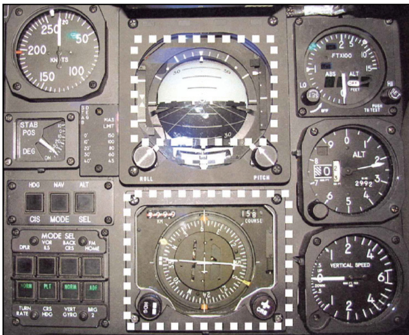
Figure 2-3. Navigation instruments on a UH-60
