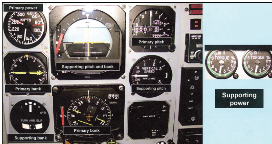
Figure 3-6. Reduced airspeed stabilized
