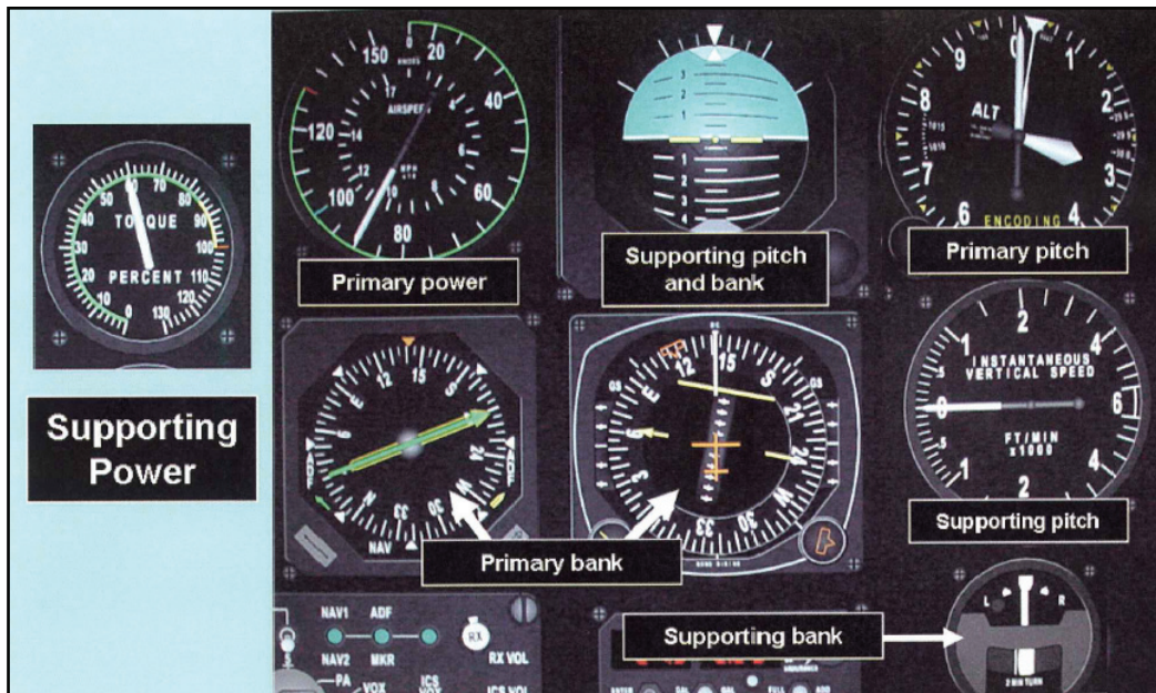
Figure 2-9. Straight-and-level flight at normal cruise speed
