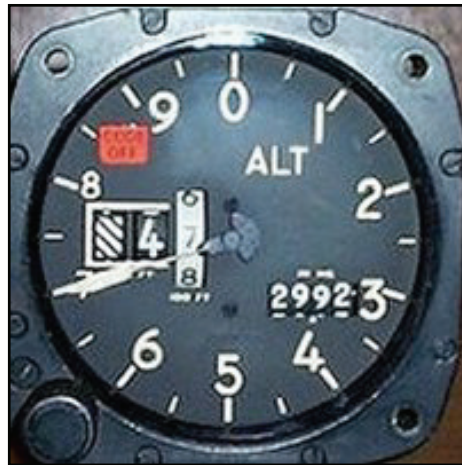
Figure 1-7. Encoding altimeter with a malfunction
