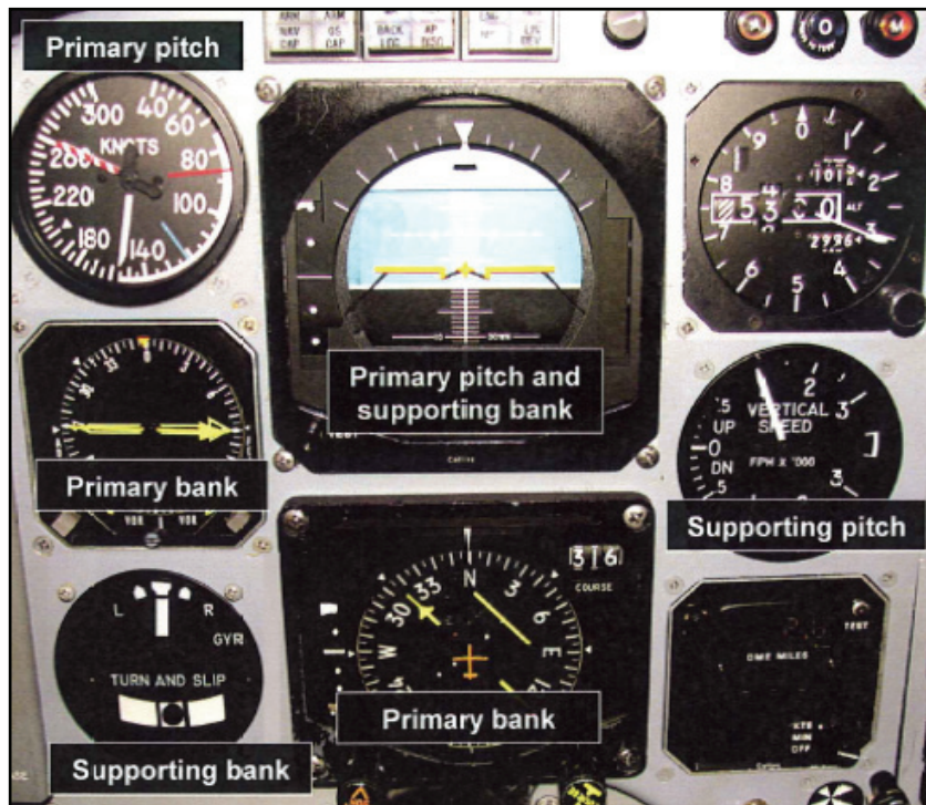
Figure 3-8. Stabilized constant airspeed climb
