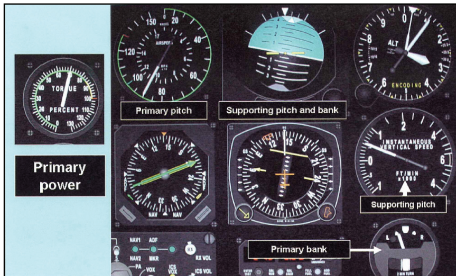
Figure 2-16. Stabilized left climbing turn, constant airspeed
