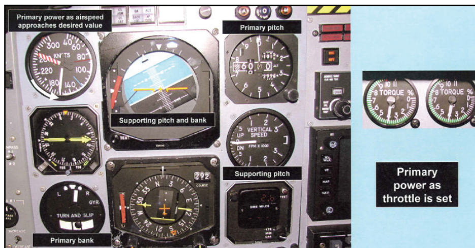
Figure 3-15. Change of airspeed in turn
