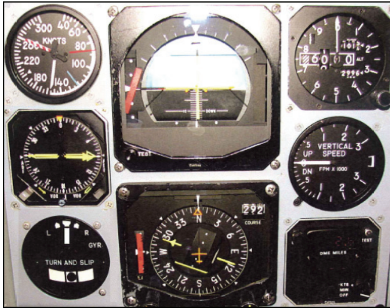
Figure 3-1. Pitch attitude and airspeed in level flight
