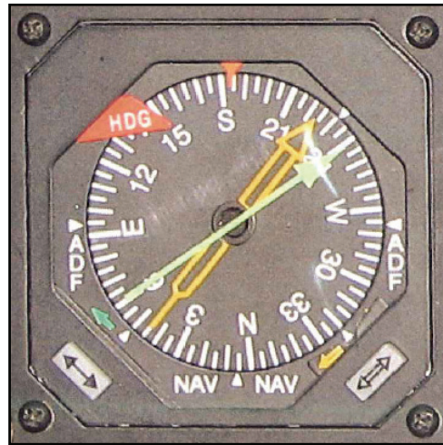
Figure 1-16. Radio magnetic indicator
