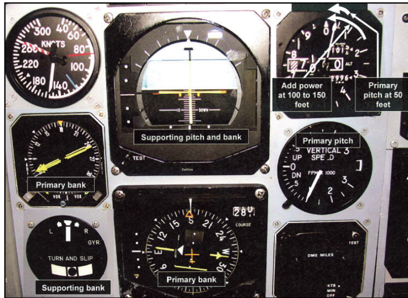
Figure 3-12. Level-off at descent airspeed
