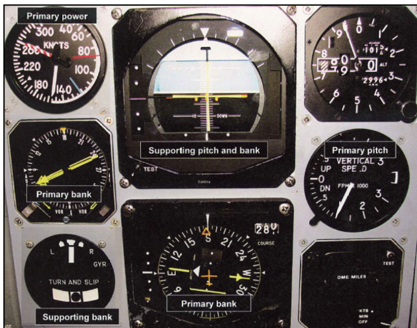
Figure 3-11. Constant airspeed descent, airspeed high—reduce power
