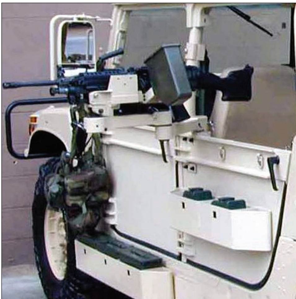
Figure K-2. Commercially produced HMMWV armored half-door and double-articulating, swing-arm mount for crew-served weapons.
