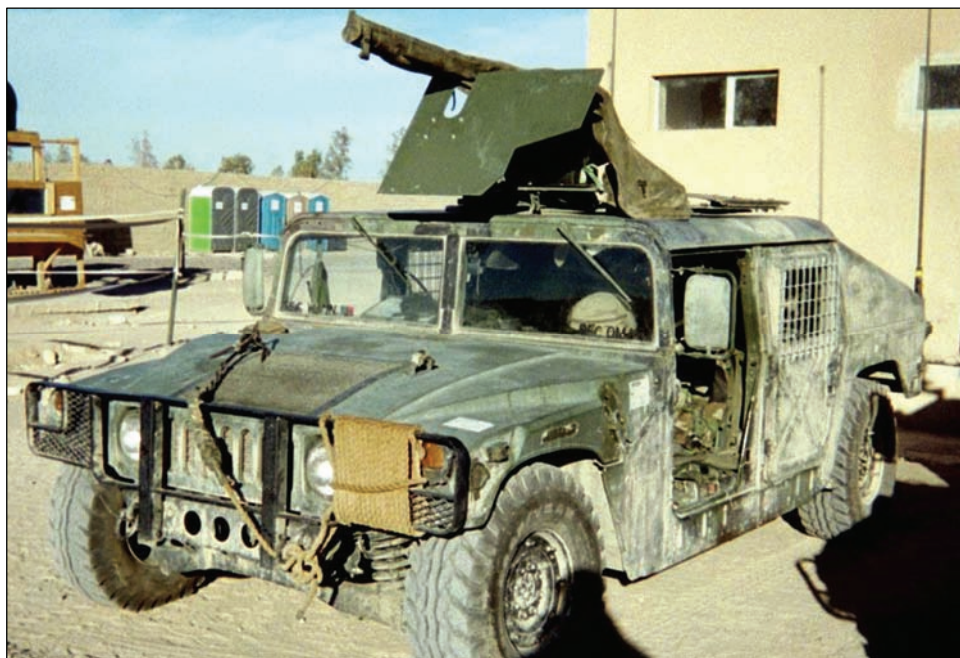
Figure K-1B. Army-issue, roof-mounted, gun-ring armor.
