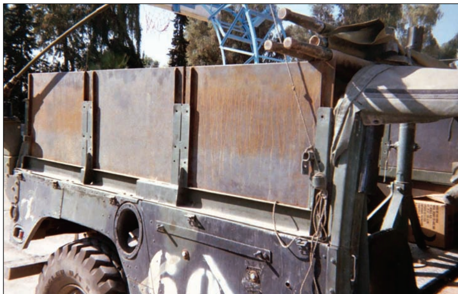
Figure K-12. Unit-installed steel armor.
