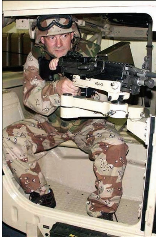
Figure K-5. Commercially produced version of an outboard-facing rear passenger seat and double-articulated swing arm for crew-served weapons.
