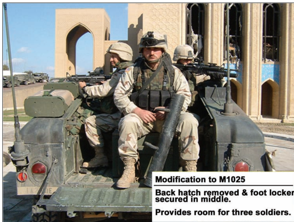
Figure K-4. Modified M1025 (turtle-shell HMMWV).
