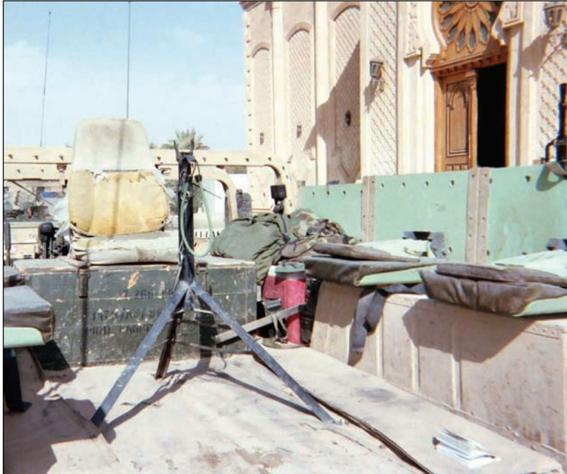
Figure K-10. Unit-produced tripod and modified armor.
