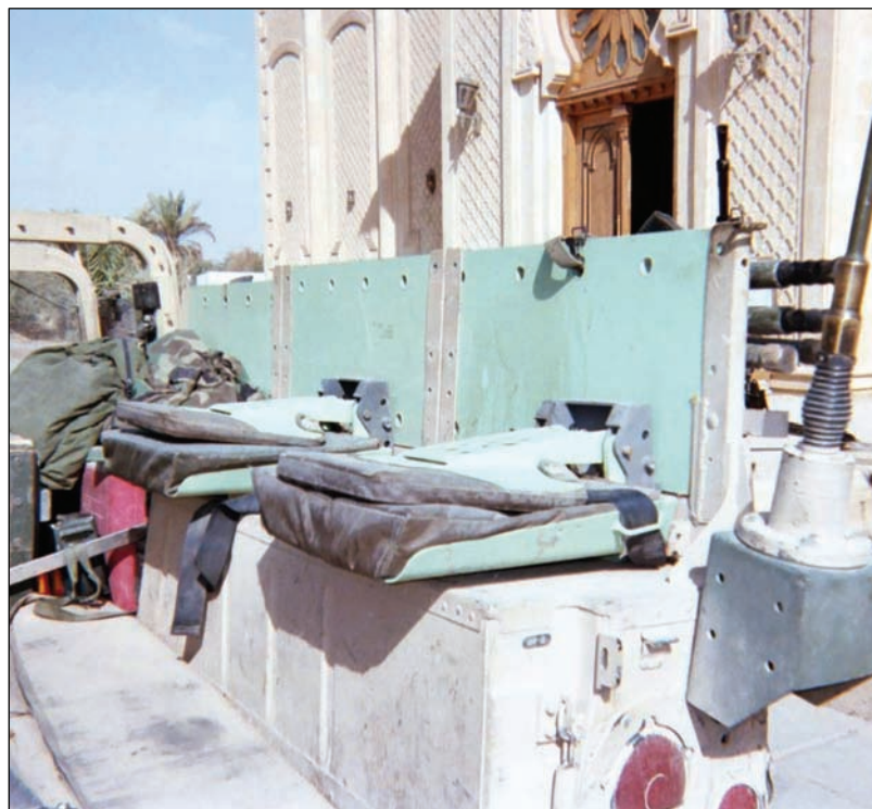
Figure K-11. Closeup of sections of Bradley fighting vehicle spall liner armor applied to exterior of cargo bed.
