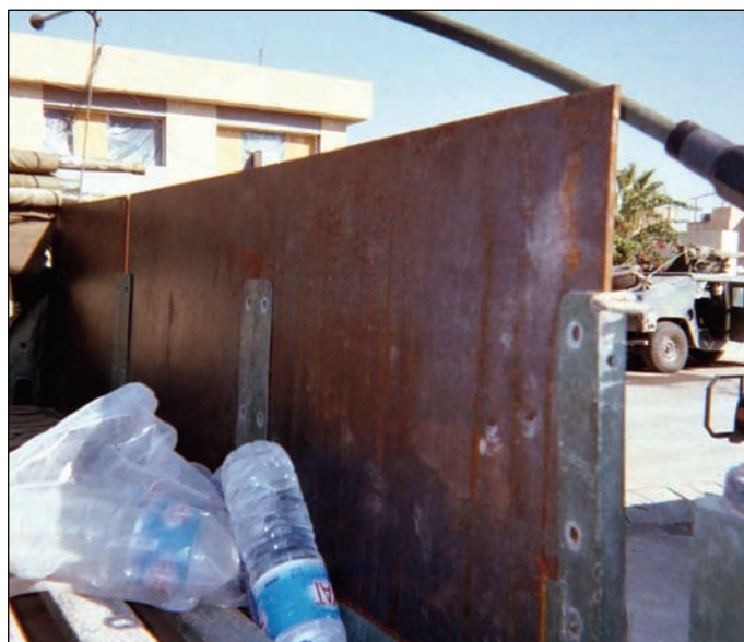
Figure K-13. Closeup, reverse-angle view of unit-fabricated and -installed steel plate armor.
