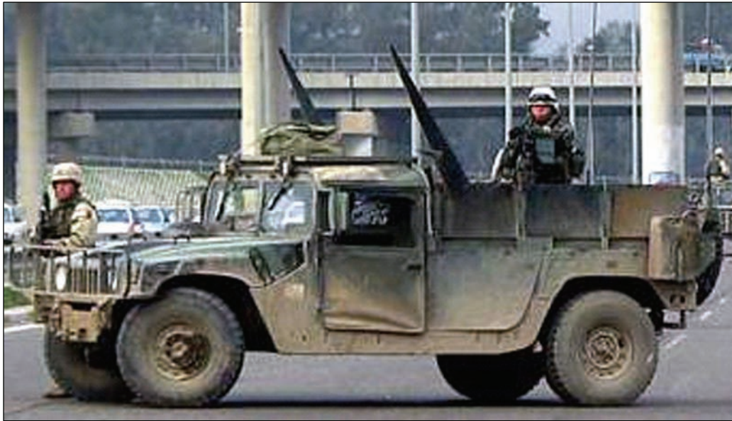
Figure K-7. Unit-installed wire cutters and wire guards.
