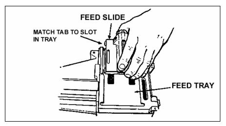
Figure 2-23. Feed slide assembly.
