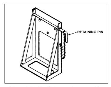
Figure 3-18. Bracket mounting assembly.
