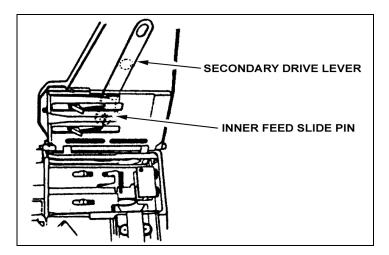
Figure 2-24. Installation of the secondary drive lever.
