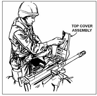
Figure 2-7. Opening the top cover assembly.
