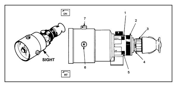
Figure G-14. Location of the AN/TVS-5 components.
