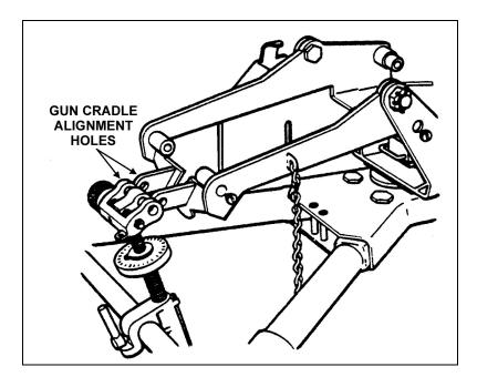
Figure 3-6. Alignment of gun cradle to T&E mechanism.
