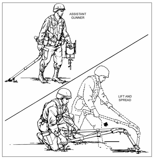
Figure H-2. Positioning the tripod.
