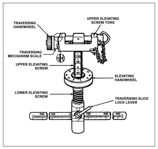
Figure 3-4. T&E mechanism.
