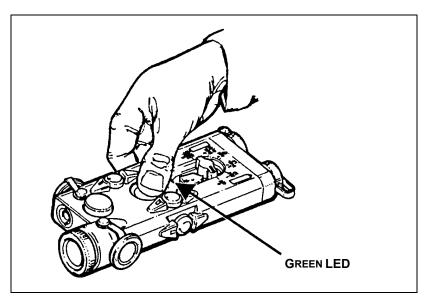
Figure G-4. Operation of the button switch.
