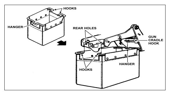
Figure 3-25. Attachment of empty case catch bag.
