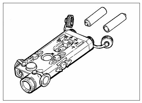
Figure G-2. AN/PEQ-2A battery installation.
