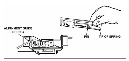
Figure 2-15. Alignment guide.
