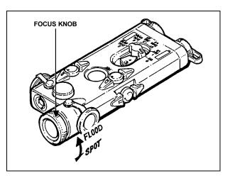
Figure G-6. Using the focus knob.
