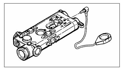
Figure G-5. Installation of the cable switch.
