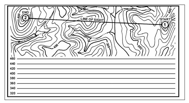
Figure 5-26. Profile line (map contour lines are 20 meters).
