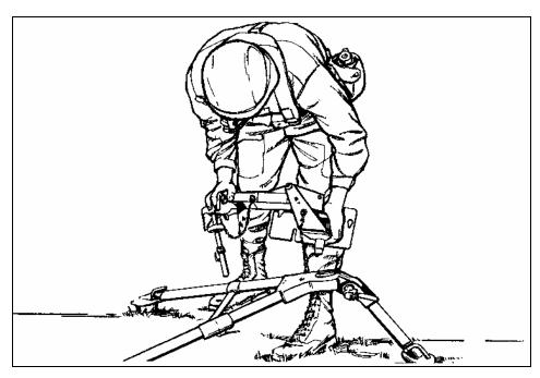
Figure H-3. Mounting the MK 19 mount on the tripod.
