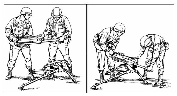
Figure H-6. Placing the MK 19 in the cradle.
