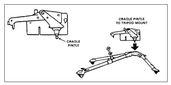
Figure 3-3. Insertion of pintle into pintle bushing.
