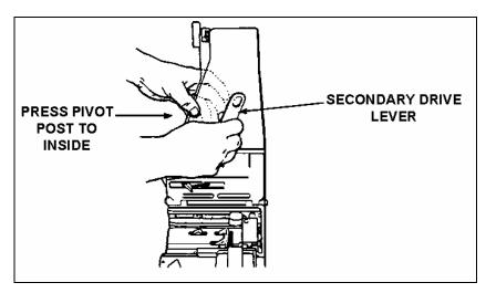
Figure 2-11. Secondary drive lever removal.
