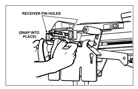
Figure 3-12. Feed throat alignment.
