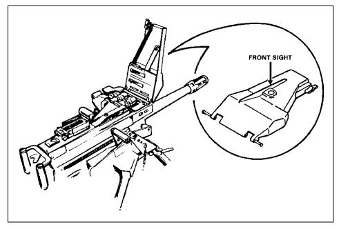
Figure 1-3. Front sight on top cover assembly.
