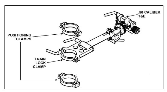
Figure 3-15. Train and elevating assembly.
