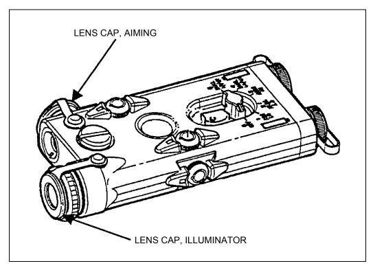
Figure G-7. Installing the lens caps.
