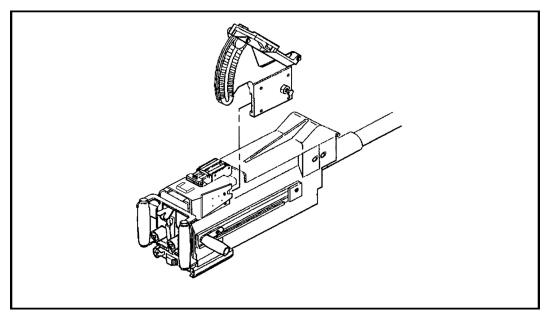
Figure G-13. Mounting the HWTS on MK 19.
