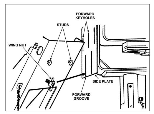
Figure 3-24. Attachment of bracket mounting assembly.
