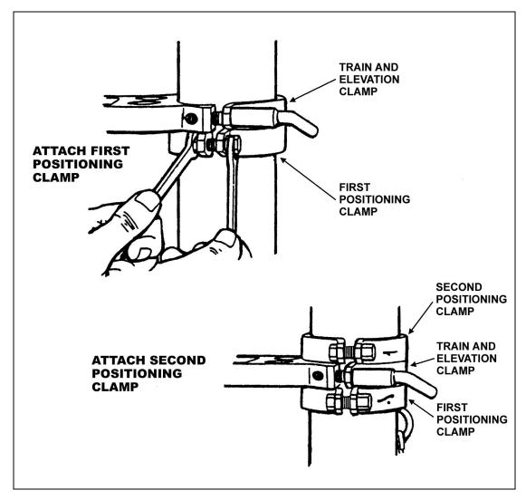
Figure 3-23. Train and elevation middle clamp.
