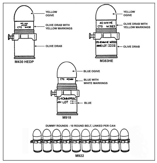
Figure 1-5. 40-mm cartridges.
