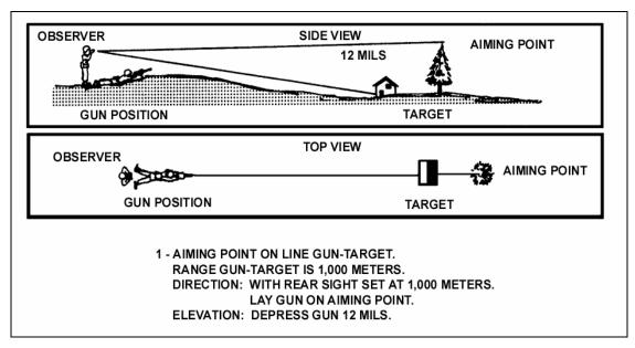
Figure 5-25. Aiming-point method for elevation.
