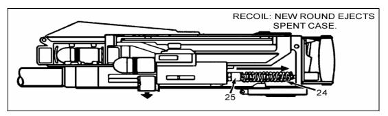
Figure 2-5. Blowback and automatic feed.
