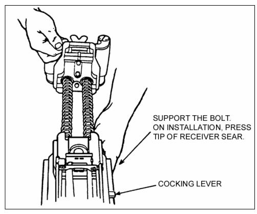
Figure 2-25. Installation of the bolt and backplate assembly.
