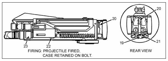
Figure 2-4. Firing cycle.
