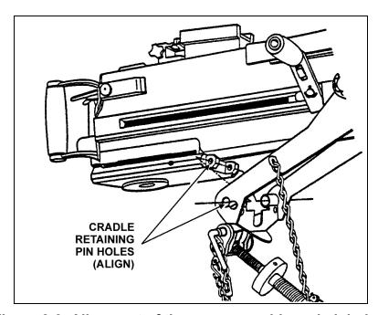
Figure 3-9. Alignment of the sear assembly and pinholes.
