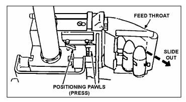
Figure 2-8. Removal of linked rounds from feeder.
