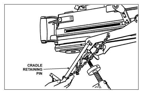
Figure 3-10. Insertion of the cradle retaining pin.
