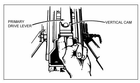
Figure 2-20. Primary drive lever and vertical cam.
