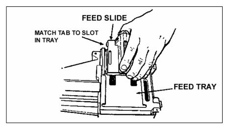
Figure 2-13. Feed slide assembly.
