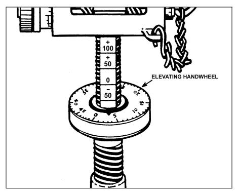
Figure 4-12. Elevating handwheel.
