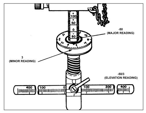
Figure 4-7. Elevation readings.
