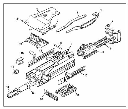
Figure 2-10. MK 19 disassembled.
