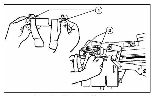
Figure 2-26. Attachment of feed throat.
