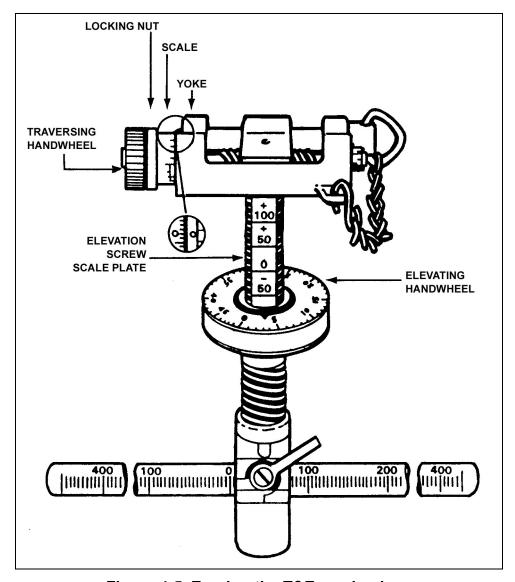
Figure 4-5. Zeroing the T&E mechanism.
