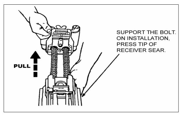
Figure 2-19. Removal of bolt and backplate assembly.
