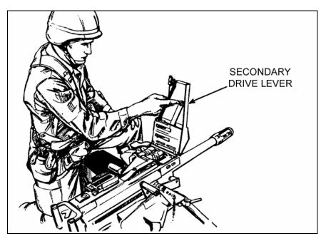
Figure 2-28. Positioning of feed slide assembly.
