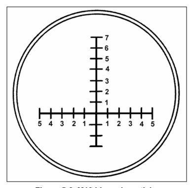
Figure 5-6. M19 binocular reticle.
