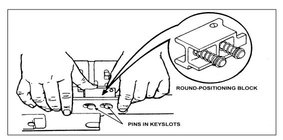
Figure 2-17. Round-positioning block.
