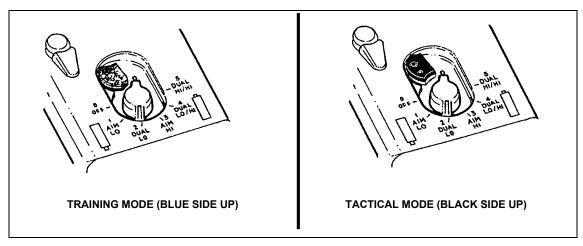
Figure G-3. Safety block installation.
