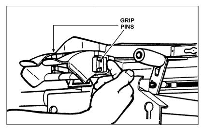
Figure 3-13. Feed throat installation.
