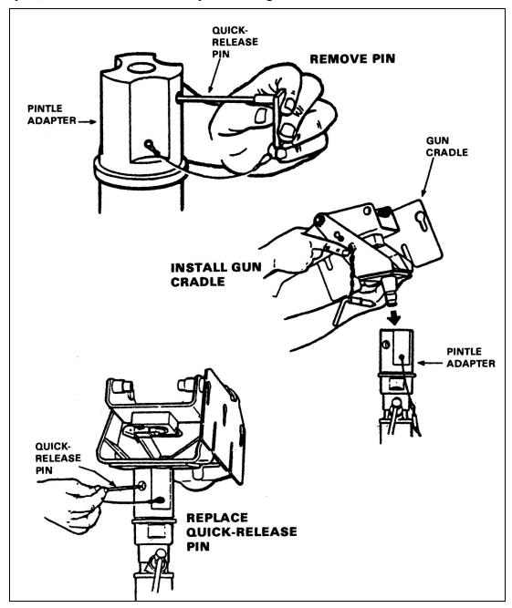
Figure 3-22. Install the carriage and cradle assembly.
