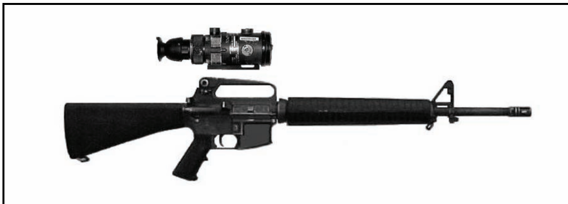
Figure 2-40. Mounting the AN/PVS-4 on an M16A1/A2/A3 rifle.
