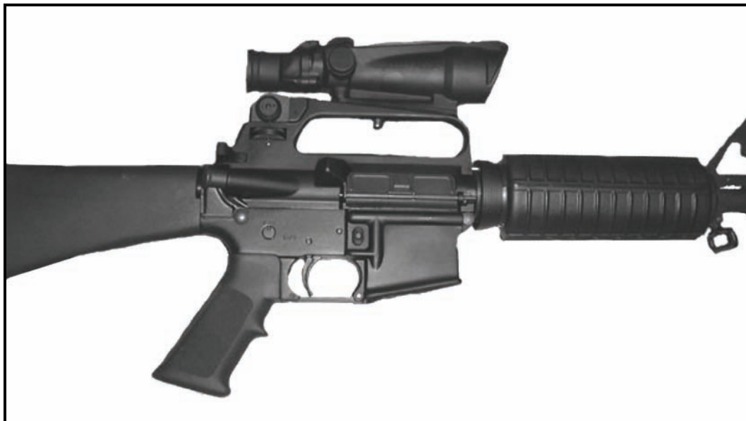
Figure 2-45. Mounting the ACOG on an M16A1/A2/A3 rifle.
