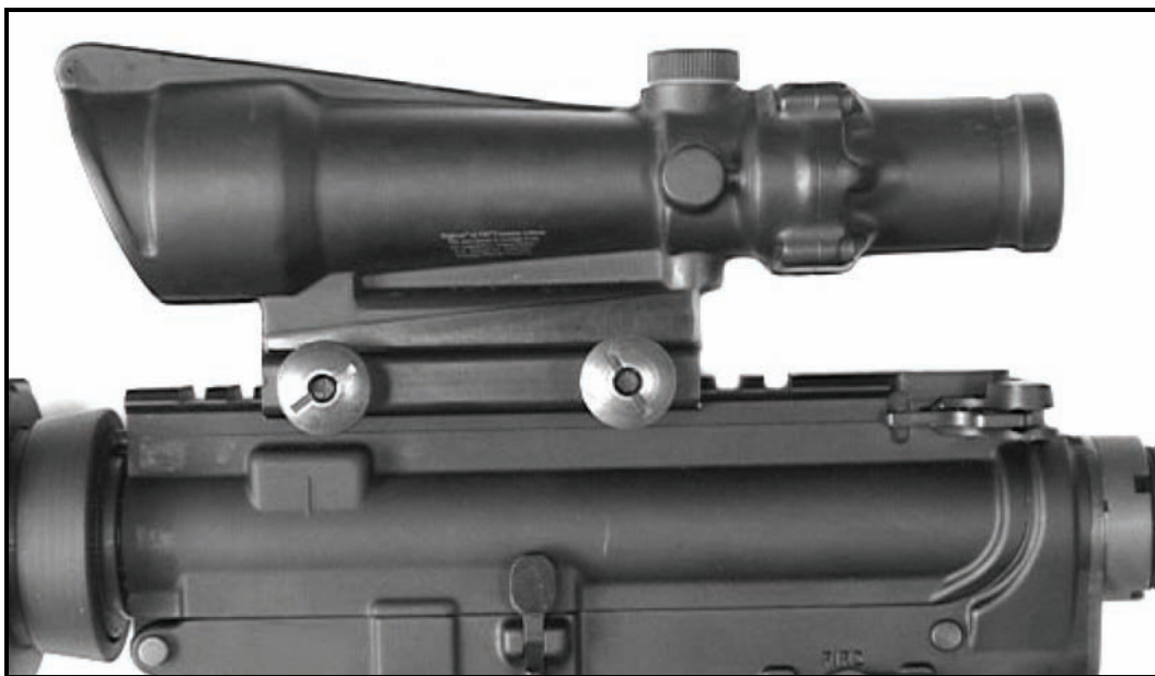
Figure 2-44. Mounting the ACOG on M16A4 rifle and M4 carbine.
