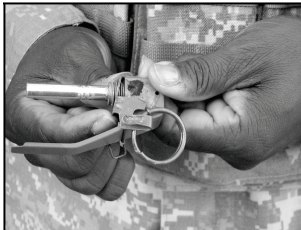
Figure A-6. Placing the confidence clip over the threaded end of the M228 fuze.
