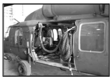
Figure 5-10. UH-60 rigged for fast roping
