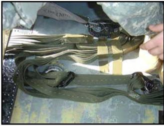
Figure 5-6. Excess cargo straps secured.
