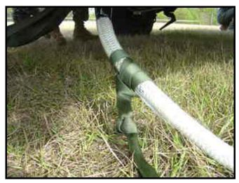
Figure 5-7. Recovery line with Prusik knot.
