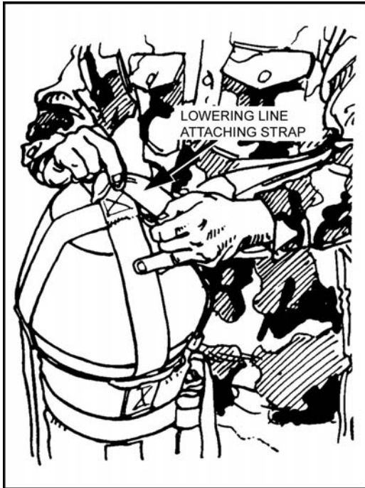
Figure 12-35. Lowering line attaching strap installed.
