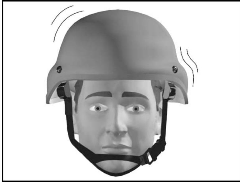
Figure 2-21. ACH too loose.
