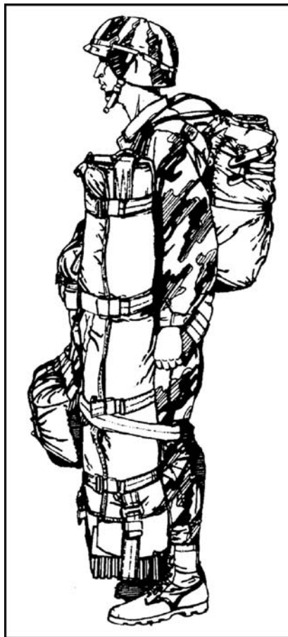
Figure 12-59. Lower tie-down tape routed around AT4JP.
