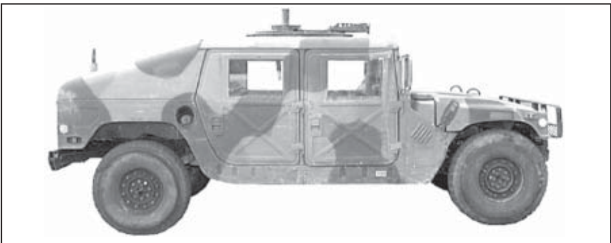
Figure 5-1. M1025/ M1121 Armament/TOW Carrier HMMWV
