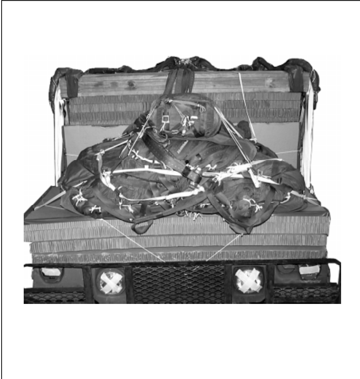
Figure 5-17. Deployment Parachutes Installed
