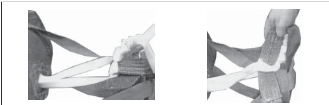
Figure 1-7. 60-inch Strap Connecting G-12 Deployment Bag to Parachute Apex Loop Completed
