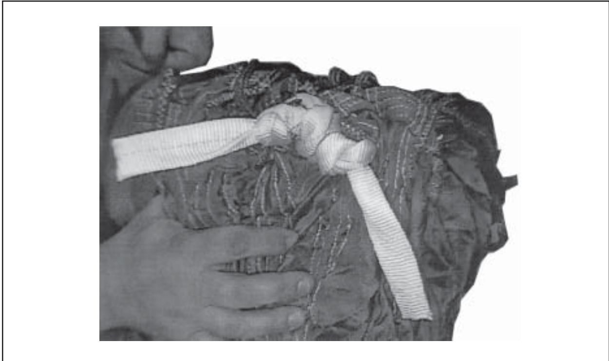
Figure 1-4. Vent Reefing Line Pulled Tight and Tied Off
