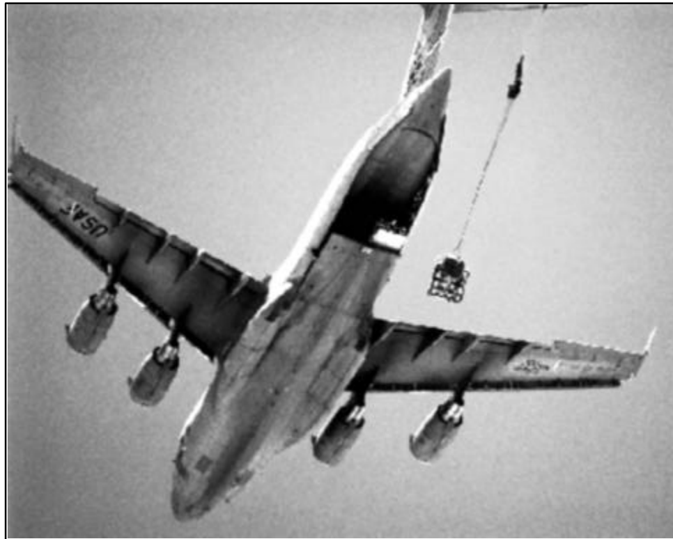
Figure 2-3. C-17 Airdrop of Pallets Using the Gravity Airdrop Method and DRAS
