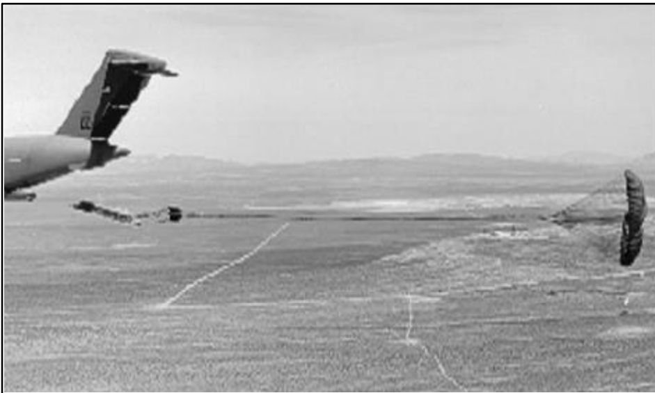
Figure 7-3. The 500-Foot Low Velocity Airdrop System (LVADS)
