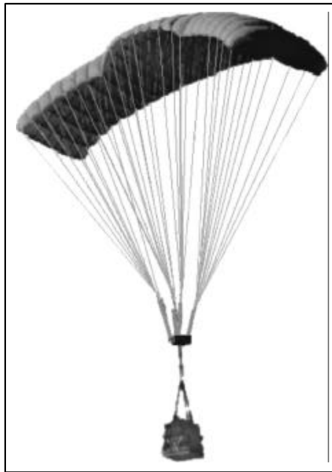
Figure 7-1. Precision Extended Glide Aerial Delivery System (PEGASYS)
