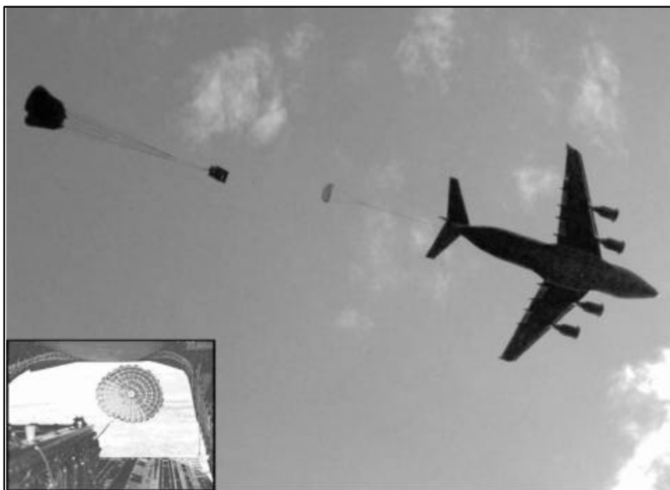
Figure 2.2. Aerial Extraction Method of Aerial Delivery
