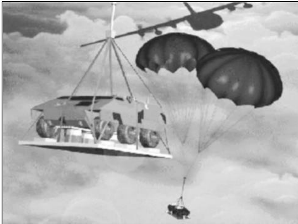
Figure 7-2. The Rapid Rigging and De-Rigging Airdrop System (RRDAS)
