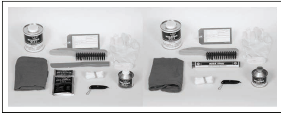
Figure 6-5. Hull and metal component repair materials
