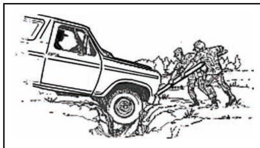
Figure 5-1. Pry bar recovery
