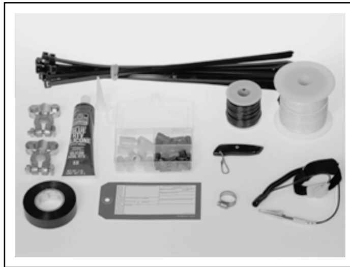
Figure 6-9. Electrical repair materials
