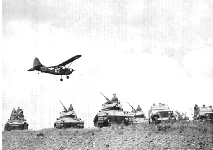
Equipment of the US Army Constabulary. Army units occupying Germany in the years after World War II were called constabulary units. Shown here are vehicles used by the Constabulary in 1946—from left to right: M8 armored car, M24 Chaffee light tank, 1/4-ton jeep. Overhead is an L-5 Sentinel observation aircraft.
