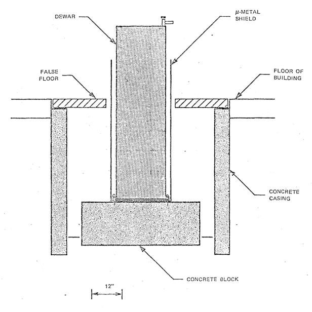
FIGURE 1 MAGNETOMETER HOUSING CONSTRUCTION
