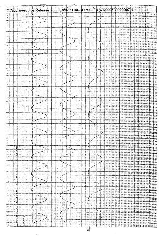
top two traces show a continuing record following termination of the experiment. The third trace was taken some time later, the increase in the period indicating the reduced rate of magnetic field decay. At various times during this and the following day when similar data with Mr. Swann were taken, the experiment was observed by numerous other scientists.
