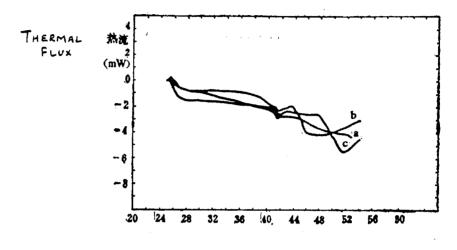
Illustration Ib: DSC curve of Specimen 2#
