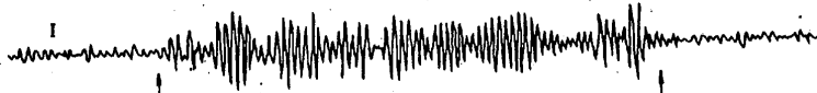
ILLUSTRATION FOUR: FIRST RECORDED MAGNETIENCEPHALOGRAPH LEFT ARROW EYES CLOSED, RIGHT ARROW EYES OPEN, 1 \times 10^{-12} TESLAR
