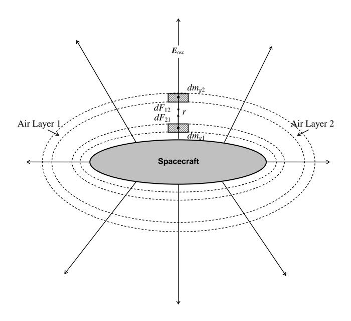
Fig. 5 – Gravitational forces between two layers of the "air shell". The electric field  $E_{osc}$  provides the *ionization* of the air.
