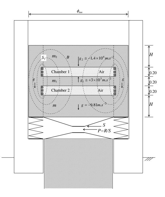
Fig. 7 – Gravitational Press
