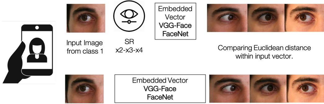
Figure 1: Block diagram of the verification framework. Top: Verification system proposed, including a super-resolution approach. Bottom: Traditional periocular verification systems.
