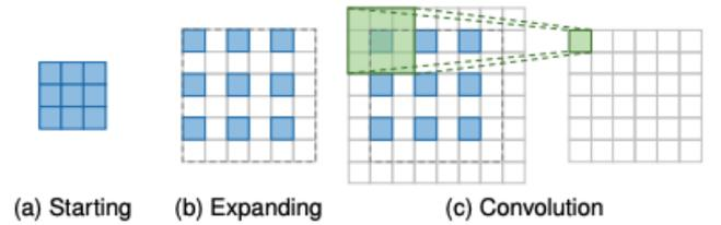
Figure 4: Transpose-convolution operation representation. (a) The starting matrix represents the input image. (b) Expanding operation adds zeros to the images in order to increase the size. (c) The convolution operation is performed again in a new resolution. Based on [5].
