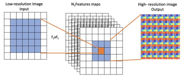
Figure 3: Pixel-shuffle convolution layer that aggregates the feature maps from LR space and builds the SR image in a single step. Based on [24].
