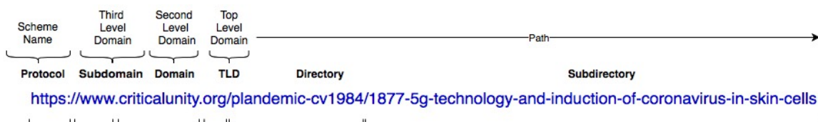
Figure 5: URL’s structure. A URL may contain mandatory (scheme, third-level, second-level, top-level domain) and optional (path) parts.
