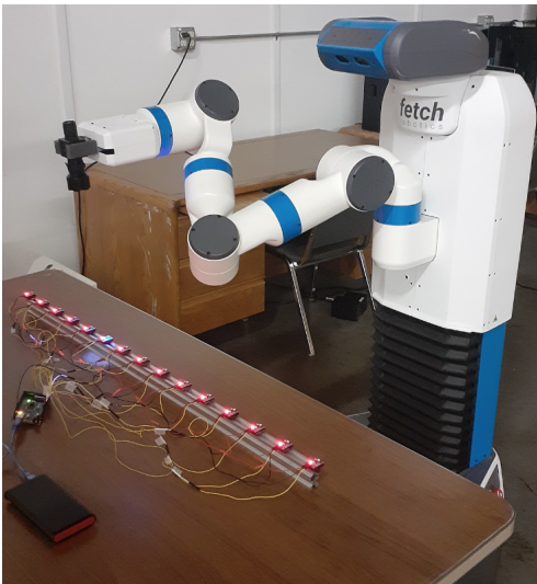
Fig. 2: A Fetch robot hovering UV flashlight above UV sensor array.
