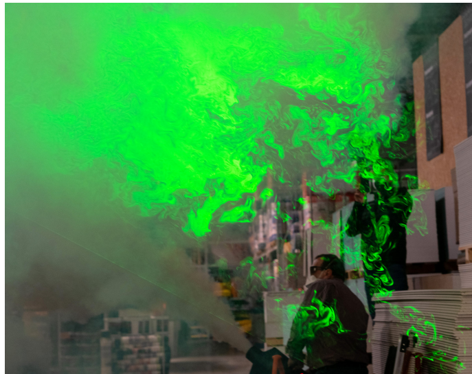
Figure 3: Flow visualization with a laser sheet reveals the turbulent vortices in the store air currents and their size distribution.
