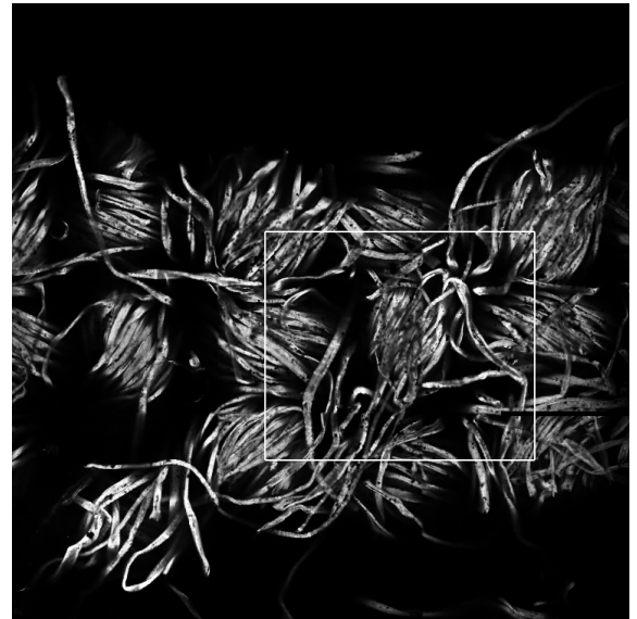
FIG. 2. Slice (number 19, starting at 0) of the confocal image of the fabric. Slice is in the xy plane. The area simulated using LB is enclosed by a white box.
