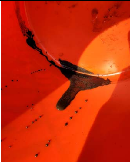
Photo 3. Sediment from turbid water from S 76304 (Madison Hill Well 1) at the beginning of well redevelopment.
