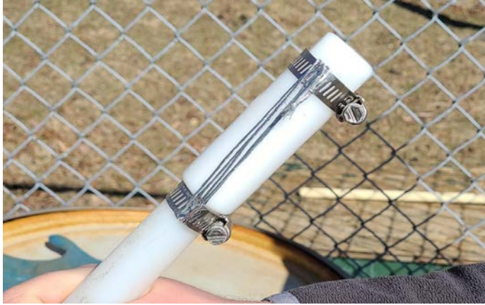
Photo 3. Check valve security, decontaminated stainless steel components, for well redevelopment at S76304 (Madison Hills Well 1).
