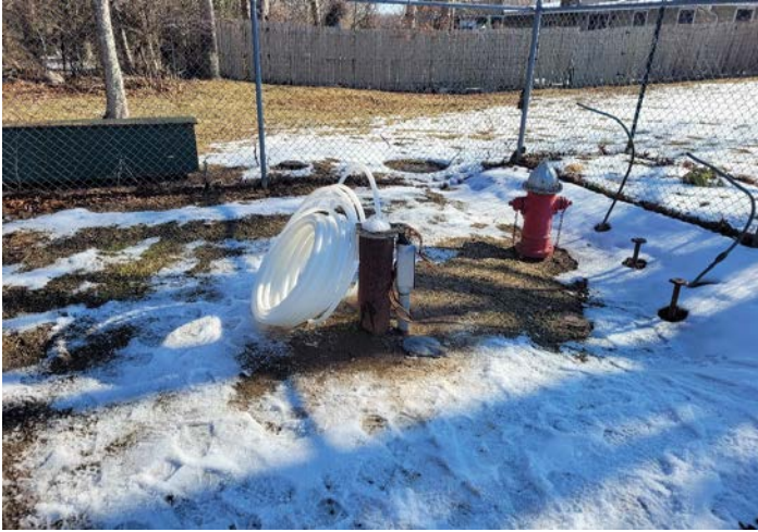
Photo 1. Preparing tubing for development/sampling; S76304.
