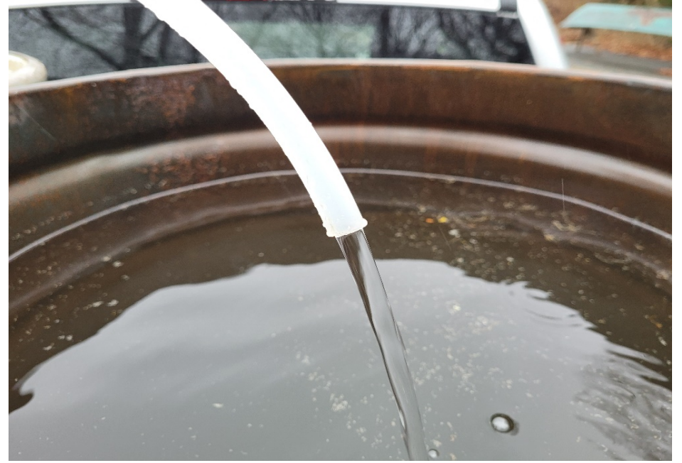
Photo 2. Purge water from S76304 (Madison Hill Well 1) at the end of the purge period; 0.62 NTU, steady 1 gpm discharge rate.
