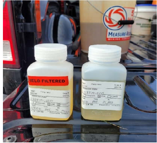
Photo 2. Recurrence of discoloration of hexavalent chromium samples once the buffer solution was added was observed at S48579.
