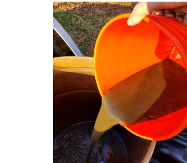
Photo 2. Turbid water from S 76304 (Madison Hill Well 1) at the beginning of well redevelopment.
