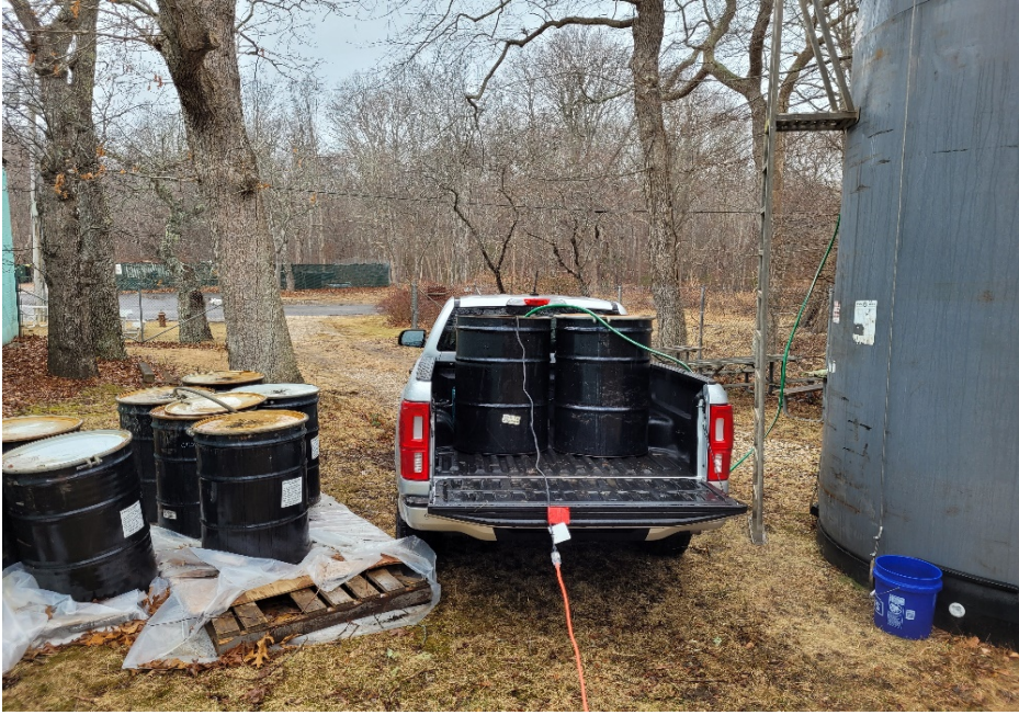
Photo 1. Purge water transfer to the frac tank at the motorpool.
