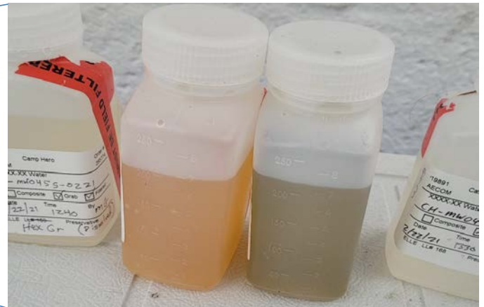
Photo 3. Discolored hexavalent chromium samples after addition of pH buffer.
