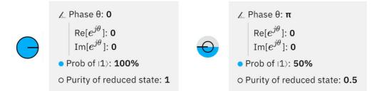
Two examples of the phase disk visualization. The first example is a  $|1\rangle$  state and the second shows the  $(|0\rangle - |1\rangle)/\sqrt{2}$  state with a nonzero relative phase.
