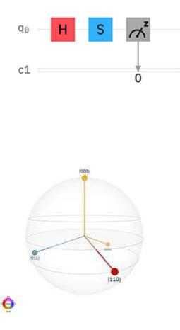
A quantum circuit and the q-sphere representing the state the circuit creates.
